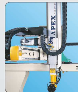
Positive servomotor drives with rack and pinion gear on vertical arm.
