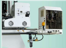
CNC control box. 6 drivers for 6 axis.
