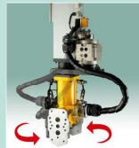
C axis pneumatic rotation device on arm (90° or 180°).
