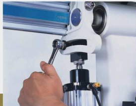
Swing out direction and angle adjusted with one screw.
